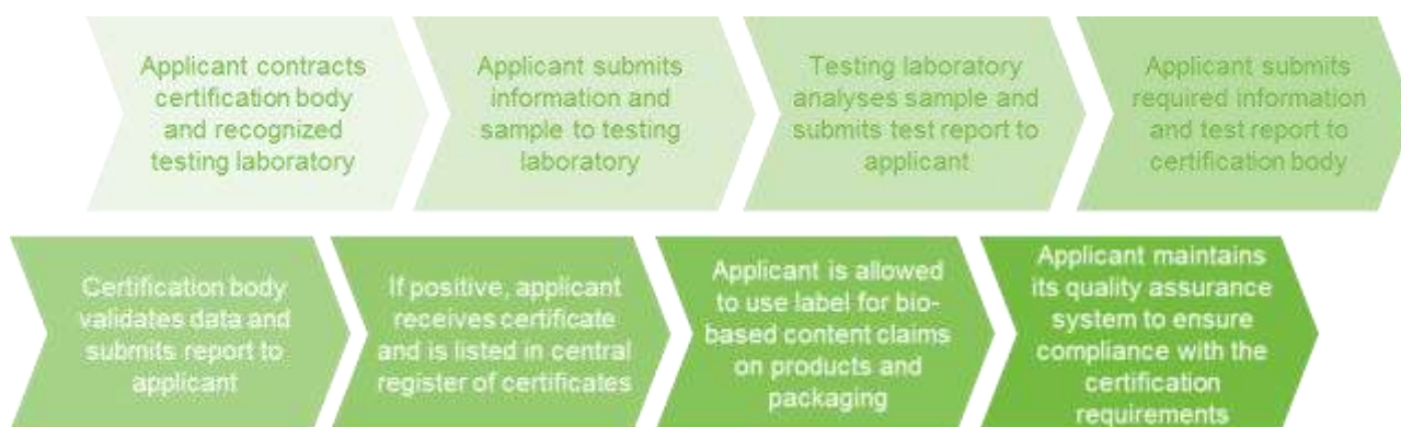
Figure 2 — Flowchart with steps to be taken by an applicant for certifying the minimum percentage of bio-based content in its product or product family
